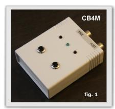
CB4M is connected with the TRX by a coaxial cable with two PL connectors. The other PL connector on CB4M is then connected to MLA feeder cable. If one uses more MLAs switched by an antenna switch, then one CB4M can be used to tune all of them.
